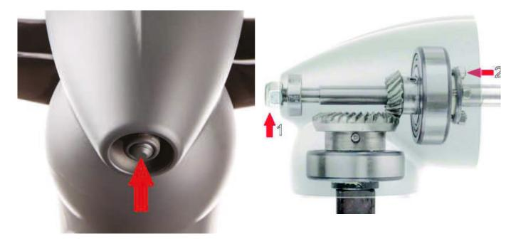
and loose or thigh the 4 grub screws (2) to "pack" the Yoke shaft and eliminated dead zone. Then, screw the 4 nuts back.
