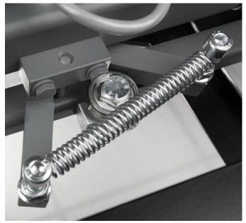
You can install or remove from 4 to 2 springs to regulate the "return to center" force.
